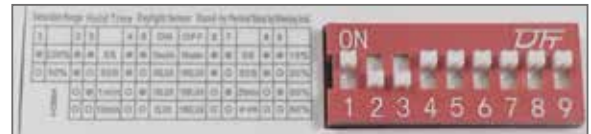
MICROWAVE SENSOR DIP Switch programmable microwave sensor with corridor function
